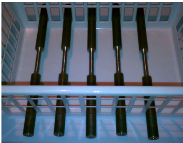
Fig. 1 Samples in holding rack prepared for immersion in the corrosion bath
