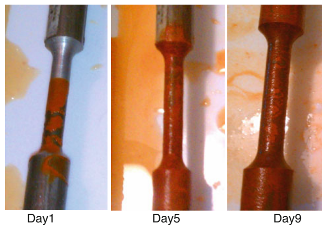
Fig. 2 NaCl and CMA samples throughout the corrosion process
